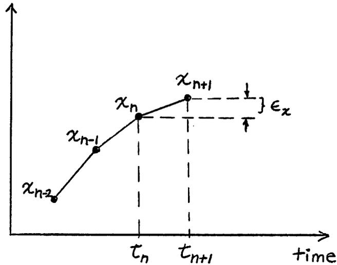
Figure 4.3 : Simple Latency Detection
