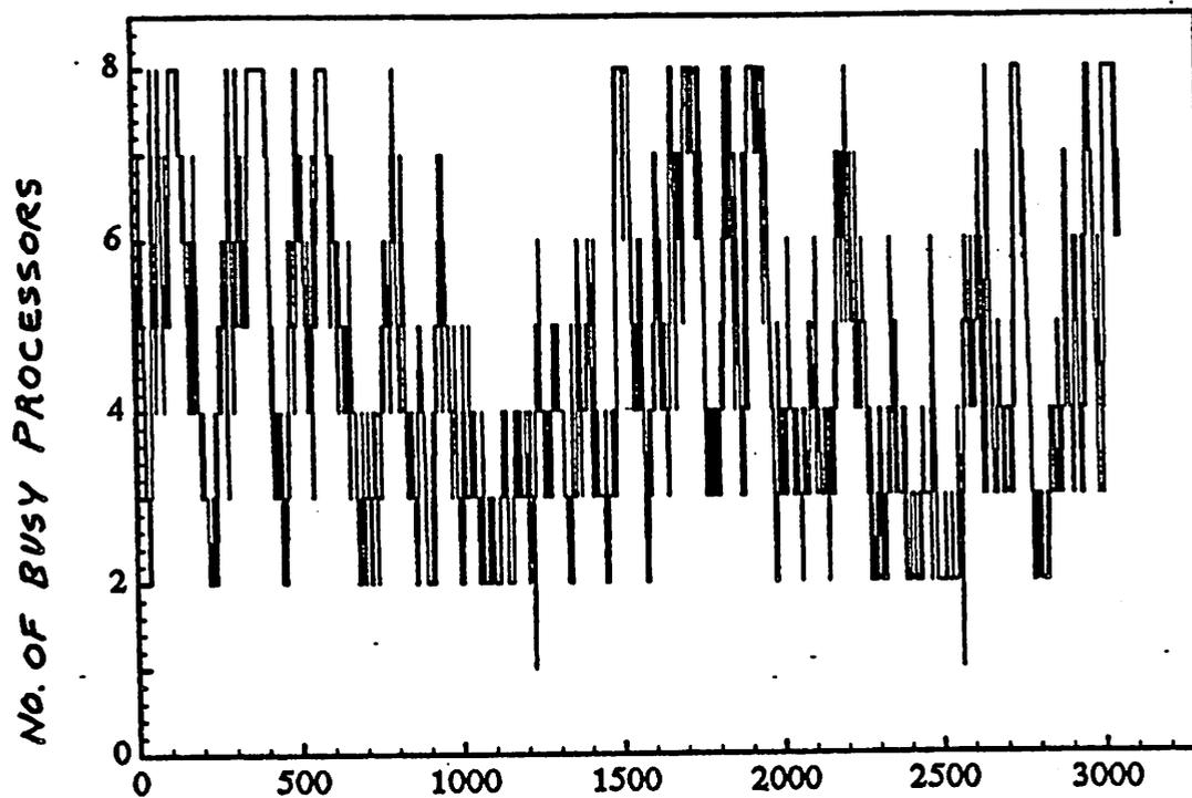
Figure 7.9 : No. of Busy Processors vs. Time for the Gauss-Seidel method
