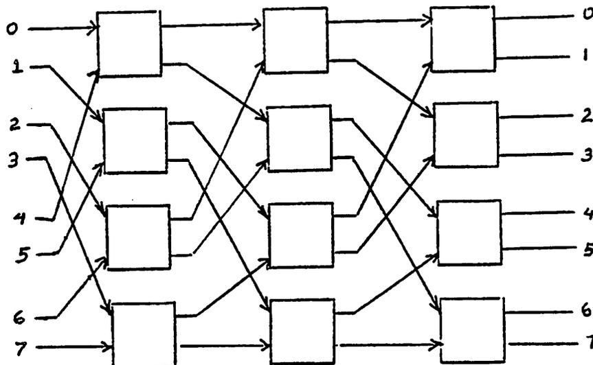
Figure 7.3 : 3-Stage OMEGA network
