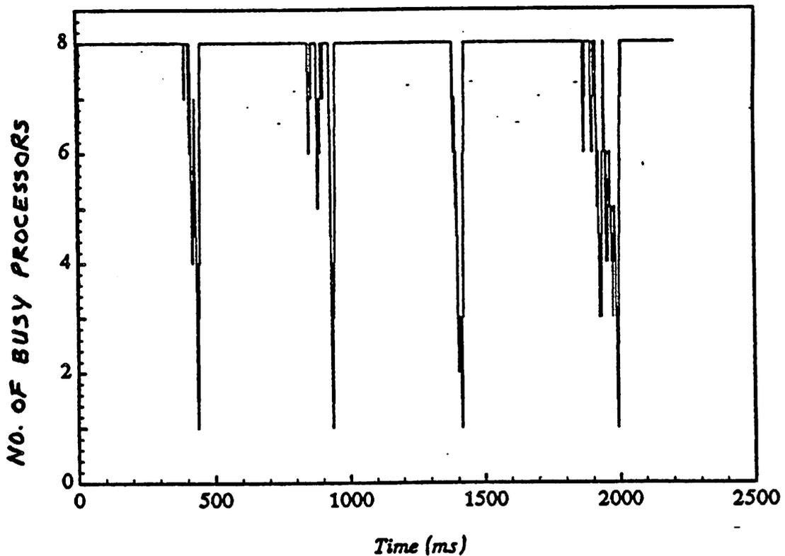
Figure 7.7 : No. of Busy Processor vs. Time for Gauss-Jacobi Method
