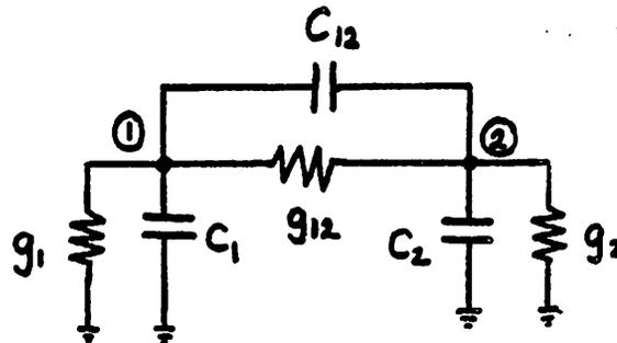
Figure 4.1 : Linear Circuit considered for Partitioning Purposes
