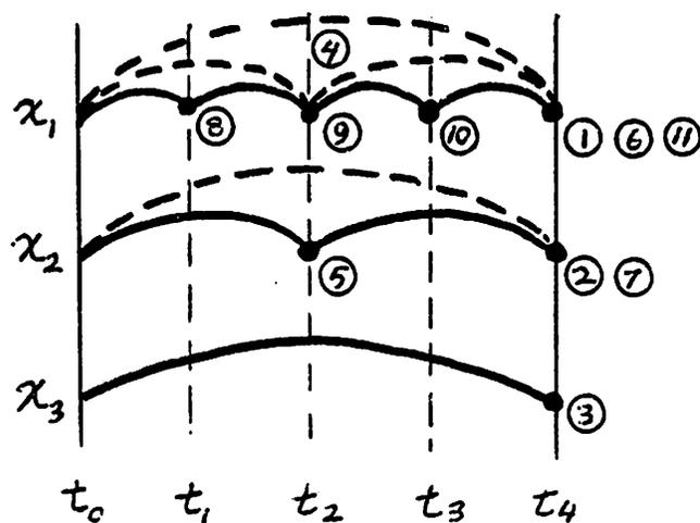
Figure 5.4 : Order of computation in the Recursive-divide-by-2 Algorithm
