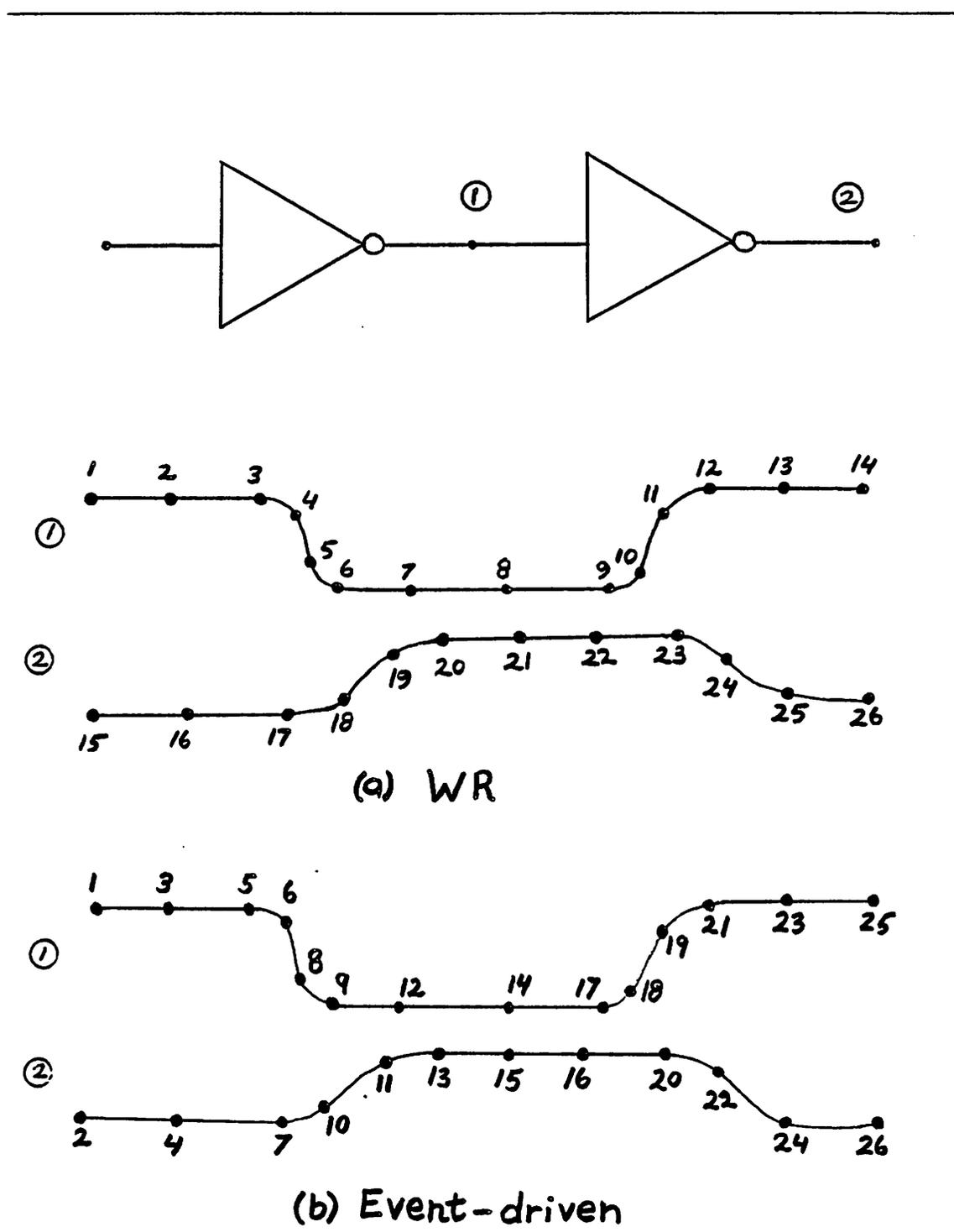
Figure 5.1 Order of Computation for WR and Event-driven Approaches
