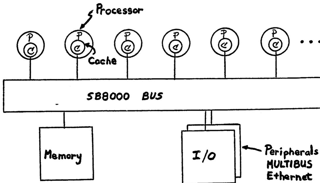
Figure 7.1 : Architecture of the Sequent Machine
