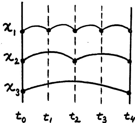
Figure 5.2 : Recommended Step sizes for a Multirate Integration Method
