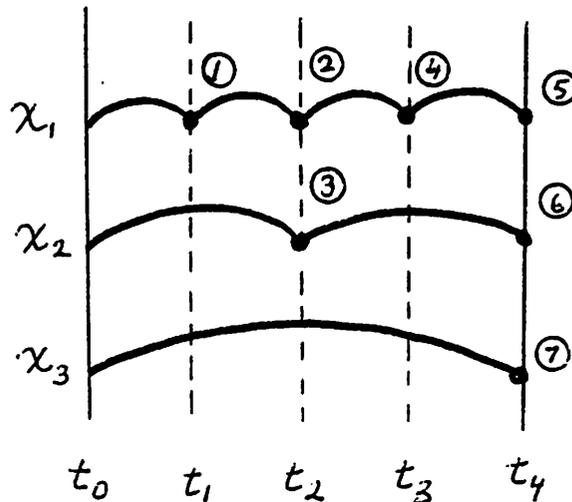
Figure 5.3 : Order of computation in the Smallest-step-first Algorithm
