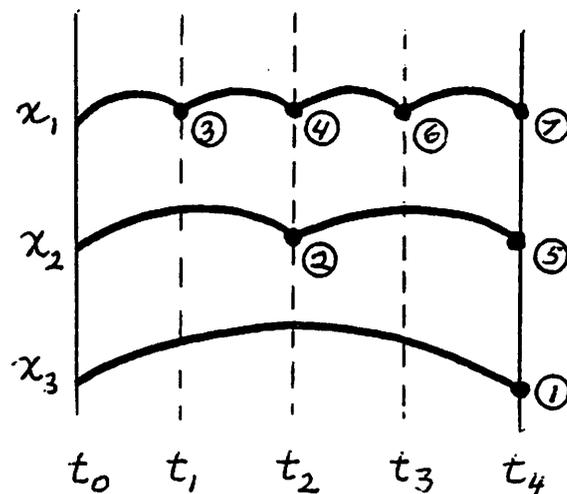
Figure 5.5 : Order of computation in the Largest-step-first Algorithm
