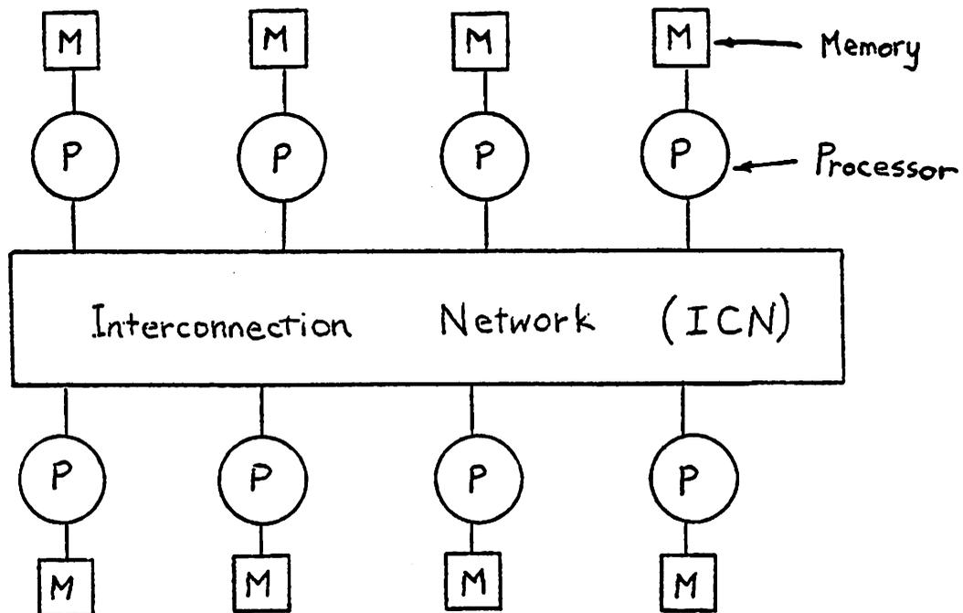
Figure 7.2 : Architecture of the BBN Butterfly
