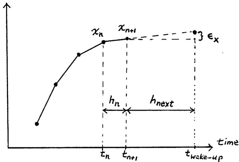
Figure 4.6 : Wake-up Mechanism
