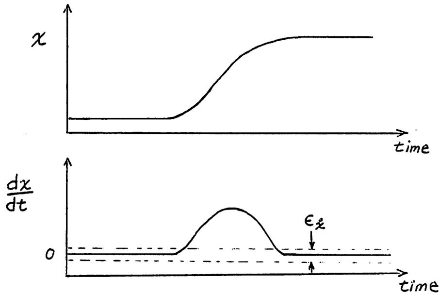
Figure 4.5 : Variable Step Latency Criterion Based on Rate-of-change
