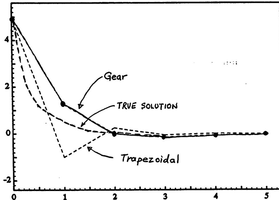
Figure 6.5 Gear-2 Integration Method
