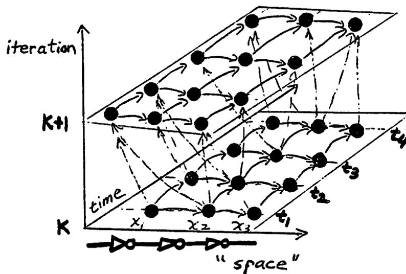
Figure 7.13 : Time-Space Model of Computation
