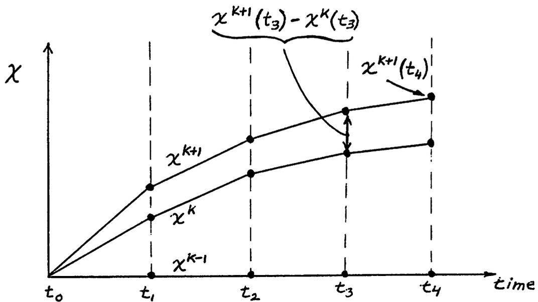
Figure 6.1 Waveform-Newton Iterations
