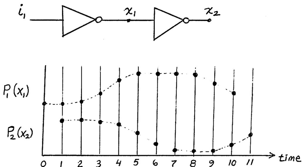
Figure 7.11 : Time Point Pipelining Example
