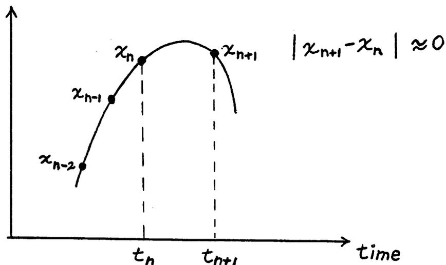
Figure 4.4 : Potential Problem in Latency Detection
