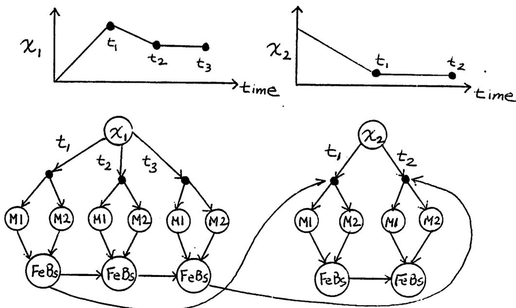
Figure 7.12 : Task Precedence Graph for 2-stage Inverter Chain Example
