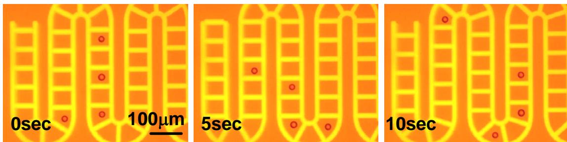
Fig. 4-2 A dynamic optical conveyer that transports multiple particles. The  $20\text{-}\mu\text{m}$  polystyrene particles are transport in a speed of  $20\ \mu\text{m}/\text{sec}$ .
