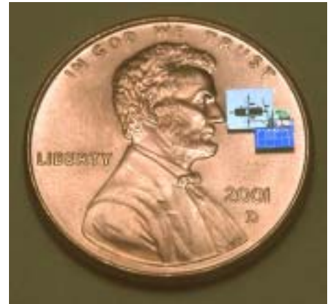
One "Smart Dust" module neatly covers the date on a U.S. penny
