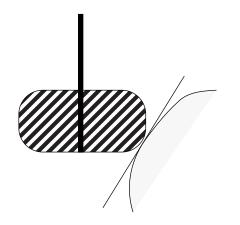
One of the machine's cutting heads cuts a toroidal excavation. The machine must lower the head to barely touch a support-plane of the work to be produced from a metal blank. To position the head requires the solution of a quartic equation. According to p. 2 of http://en.wikipedia.org/wiki/Quartic\_function as of 12 June 2014, ... "Over 10% of the computational time in a CAM system can be consumed simply calculating the solution to millions of quartic equations."
