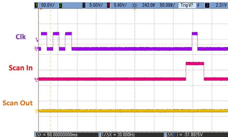
Fig. 4.18 Digital signals outputted from DB25 port used to control the scan-chain.
