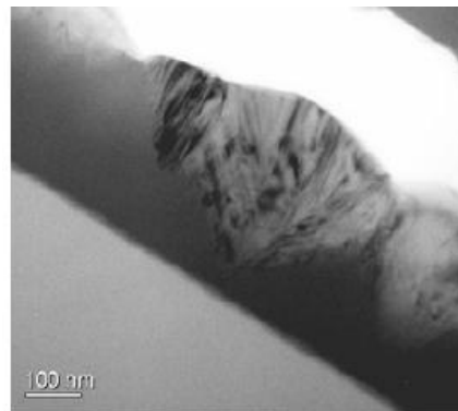
Fig. 4.5 HR-XTEM of a ~500 nm-thick poly-Si 0.4 Ge 0.6 deposited using the stress gradient optimized deposition recipe. Note that the film is only partially polycrystalline with significant thickness variation (adapted from [7]).
