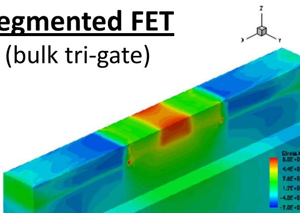
Contact etch stop liner is assumed to be a 30nm-thick silicon nitride with 2GPa tensile stress
