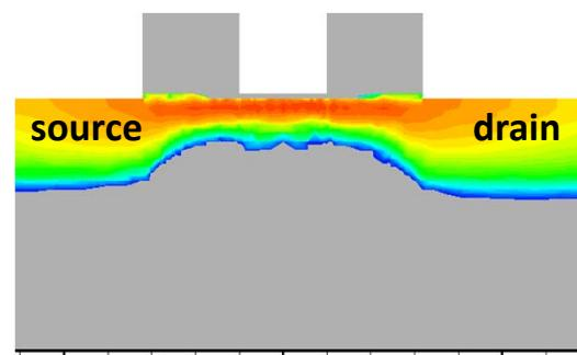
Retrograde channel doping (ground plane) is insufficient!
