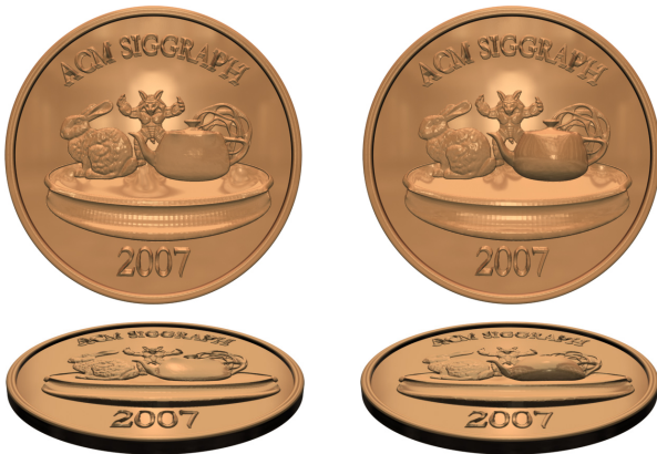
Figure 4: Selective scale modification. Left: A bas-relief of a still life in bronze under natural environment illumination. Right: Scale emphasis of a scene element. Corresponding height fields are shown underneath.
