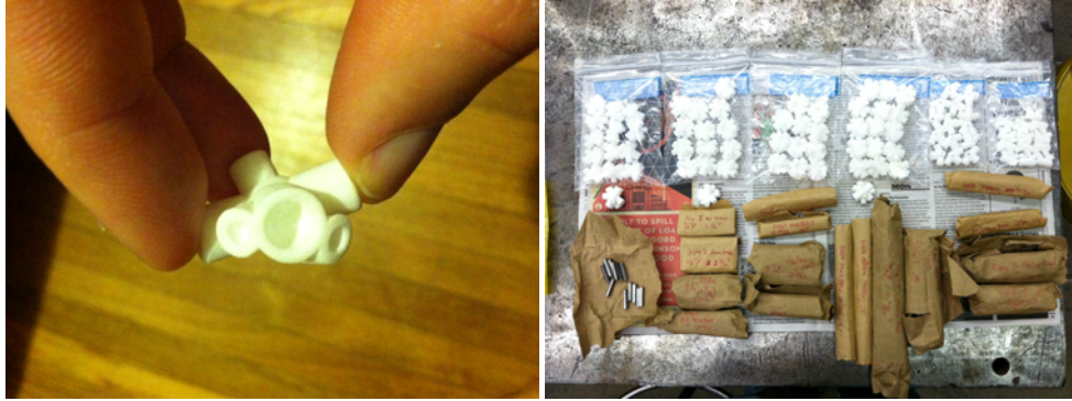
Figure 10: Joints contained leftover nylon powder that had to be removed with a paperclip. The assortment of finished parts was laid out prior to assembly.
