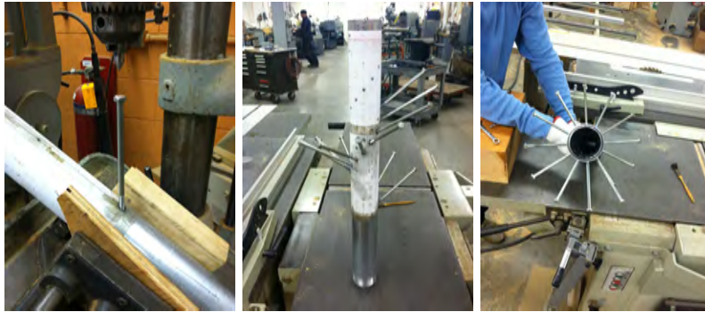
Figure 8: Drill press was set up at an angle of 32 degrees to drill and tap holes. Fit was tested with 1/4" bolts. Alignment of bolts was accurate. Bolts were then cut to length to produce the innermost ring of rib rods.
