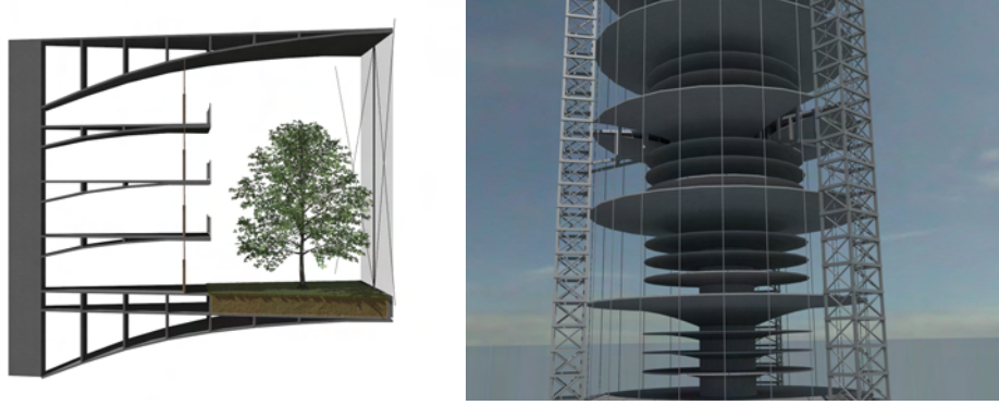
Figure 2: Structure consists of floors where the concrete floor deck is supported on a curved concrete shell. The shell is revolved around a center column, with services in external structures at the outer rim.
