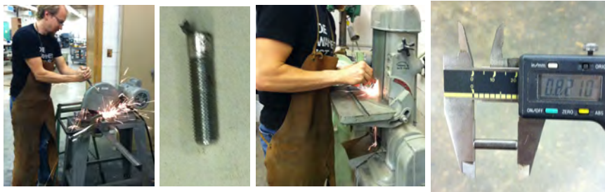
Figure 9: Rods were cut, leaving metal flash. This was ground down, and the ends were beveled. Final rod length was checked with digital calipers. Rods deviated upwards a maximum of 20 mils from the target length, and downward a minimum of -5 mils.
