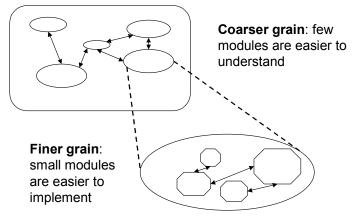
Figure 2. An illustration of hierarchical decomposition.
