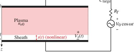
• Series resonance (capacitive sheath + inductive plasma)
