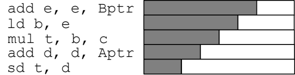
Figure 4: Active Instruction Window. The resulting instruction window at a certain point in time when executing the code in Figure 2. This example uses a vlen of 64. A grayed out box indicates that corresponding \mu T has committed that instruction.
