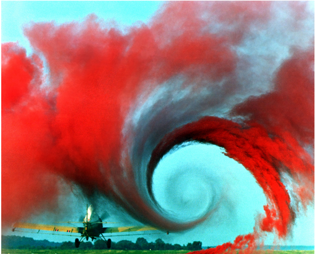
Figure 10.1: Turbulence in a vortex from the tip of an airplane wing tracked with the help of colored smoke. [Image by NASA Langley Research Center, released into the public domain.]
