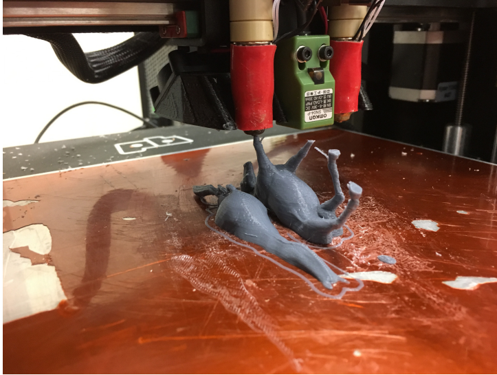
Figure 2.3: A model of a horse being printed by a 3D printer. [Photo by Ben Zhang, courtesy of the photographer.]
