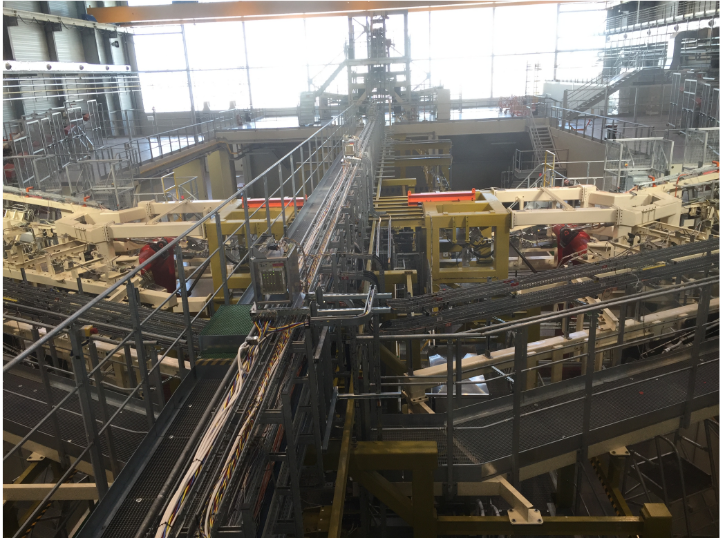
Figure 6.4: An Airbus “iron wing” prototype of an A350.
