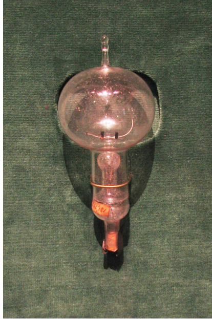
Figure 2.6: Prototype from Thomas Edison’s shop of an incandescent lightbulb with a carbon filament. [Image by Terren - Edison Light Bulb , licensed under the Creative Commons Attribution 2.0 Generic license. Lightened by the author. Original from Wikimedia Commons.]
