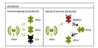
Figure 2: Broadcast Eavesdropping (left): Two of Alice's own components receive the broadcast, but so does Eve's component. Broadcast Denial of Service for Ordered Broadcasts (right): Mallory's component receives the broadcast first and prevents Alice's other components from receiving it.
