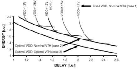
**Fig. 5.** Energy - delay tradeoff curves for different sets of optimization variables
