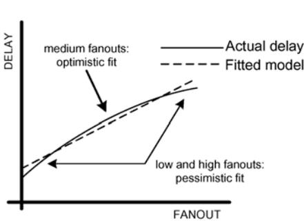
Fig. 3. Accuracy of fitted models
